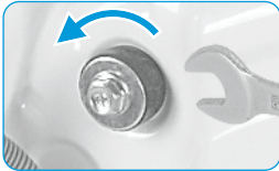
Loosen the 4 transport bolts with a spanner.
